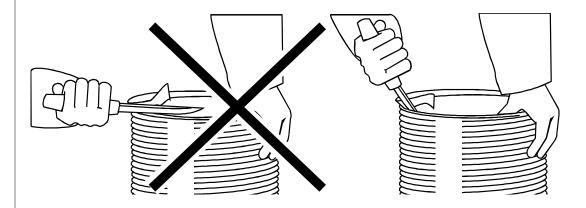
Excess plastic protection should be cut away. The elasticity in the lifting hose can be retained by cutting with the thread as shown in the right hand diagram.
