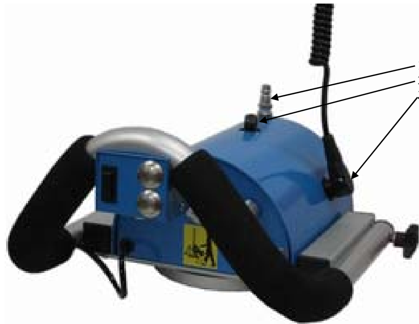
Picture 9. Gripper attachments. 1) Air attachment. 2) Loop for shackle 3) Connector to control cable.
