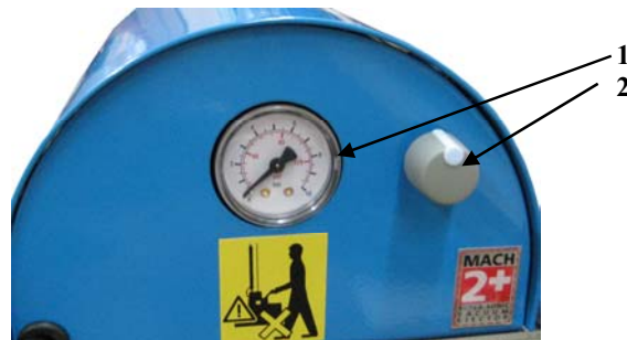
Picture 8. 1) Pressure gauge on gripper. 2) Lifting speed rheostat
